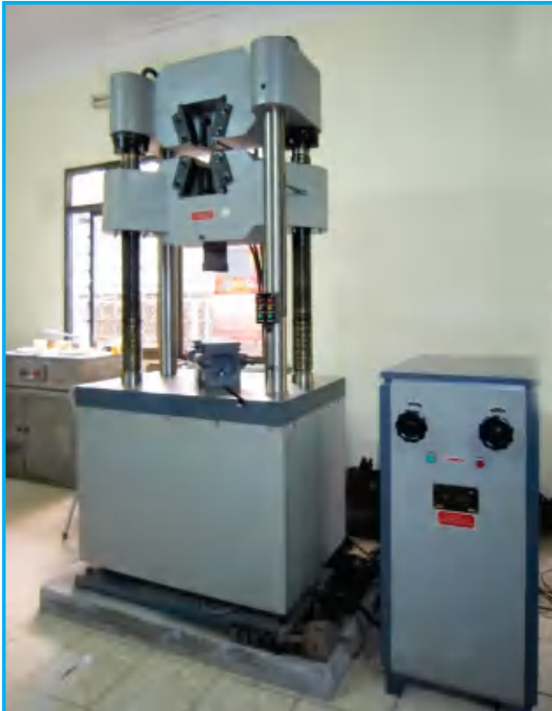
Tensile test machine for connection between ball node and bolt
