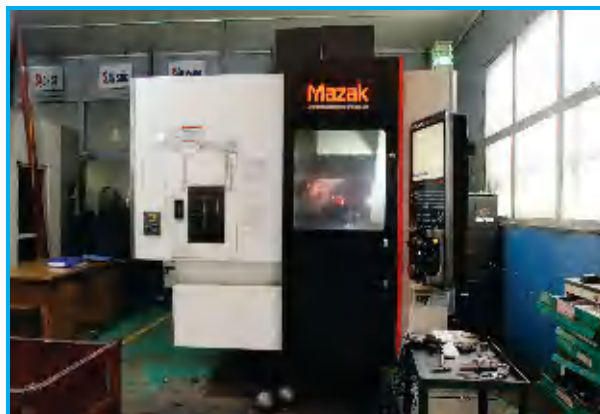
Mazak 5-Axis Machining Center for Fabricating Joint Ball
