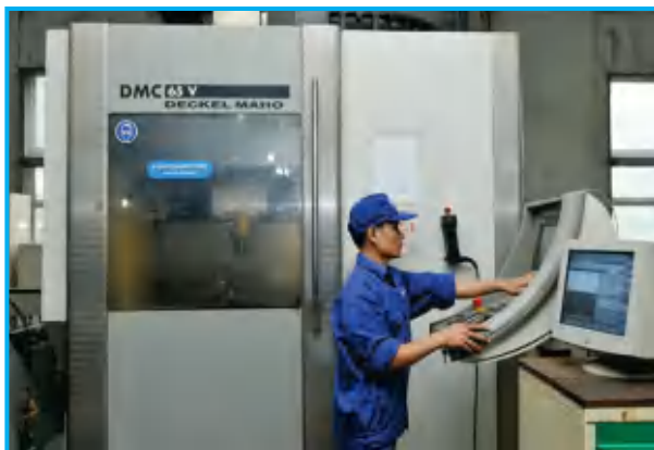
DMC 65V Machining Center for Fabricating Joint Ball
